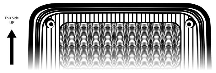
\*Light should be oriented with overlapping circles facing downward to direct light toward ground
