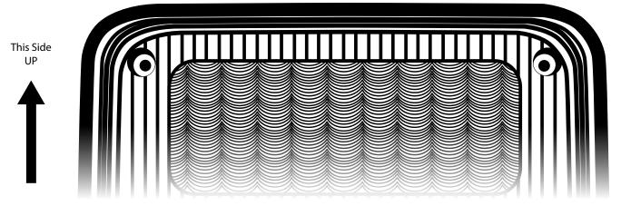
\*Light should be oriented with overlapping circles facing downward to direct light toward ground
